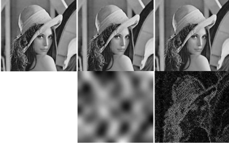
Fig. 1. Comparison of Cox scheme (Image-Independent) and IA-DCT scheme (Image-Adaptive): (a) top-left: Original image, (b) top-middle: watermarked image by Cox scheme, (c) top-right: watermarked image by IA-DCT scheme, (d) bottom-middle: Cox 's watermark and (e) bottom-right: IA-DCT 's watermark (watermarks are scaled to be visible)
