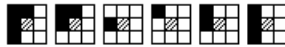
Fig. 5. Set of 3×3 template designed to be used with AWTCJ in increasing visual impact order. Only the templates that cannot cause symbol connection or disconnection are listed. Hatched pixels match either black or white pixels (note that all templates have hatched central pixels). The score of a given pattern is that of the matching template with the lowest impact. Mirrors, rotations and reverses of each pattern have the same score.
