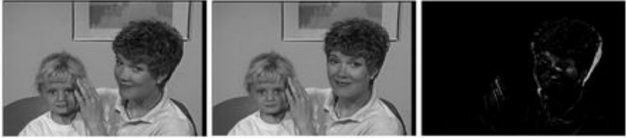
Fig. 5. Our motion parameter on two video frames. (Left): first video frame, (Middle): seventh video frame of the momdaughter sequence and (Right): the corresponding motion parameter.
