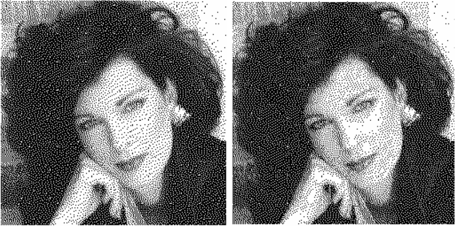
Fig. 8. The comparison results of 256 \times 256 “Debbie” image watermarking. (a) halftone image generated from DHED watermarking method (watermark rate is 0.0312 bits/pixel) (b) halftone image generated from the proposed algorithm (watermark rate is 0.0312 bits/pixel).
